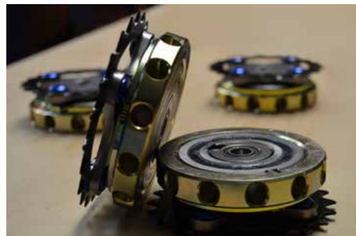
The Stieber overrunning clutch offers far more in terms of reliable performance and is now specified as standard on all Mountain Trikes.
