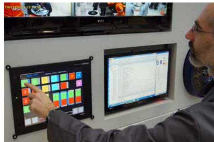
The GOT touch screen HMI displays comprehensive information on a large number of parameters such as welding gas flow, cutting gas flow, robot position, laser power, safety functions, etc.
